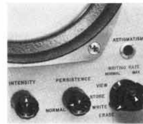
141A Oscilloscope is identical to 140A except for addition of variable persistence and storage modes
